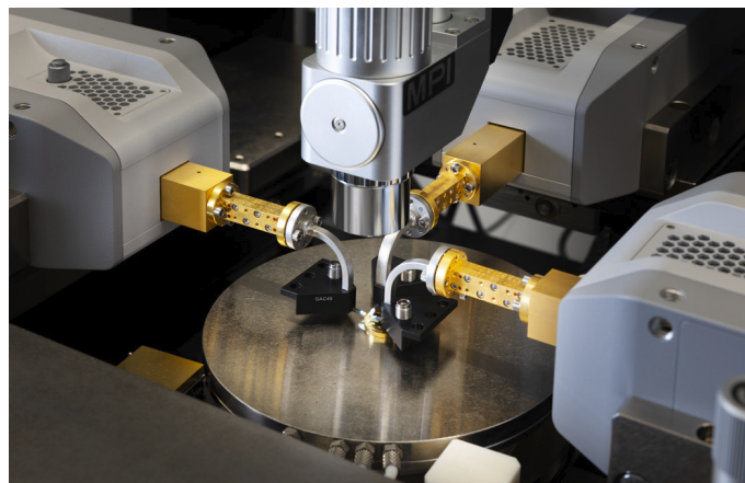
Frequency mmW converters integration on MPI THZ system platform for three-port characterization
