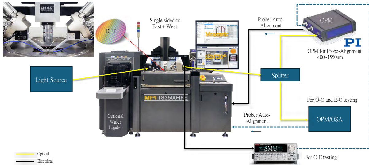
Fig. 5: Default PIC probe system configuration
