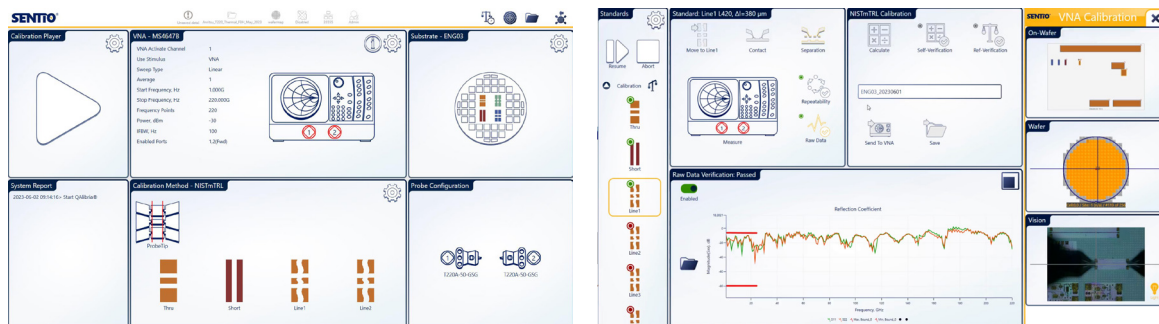
Fig. 4: QAlibria® Dashboard configured for the NIST mTRL calibration with custom on-wafer standards.
