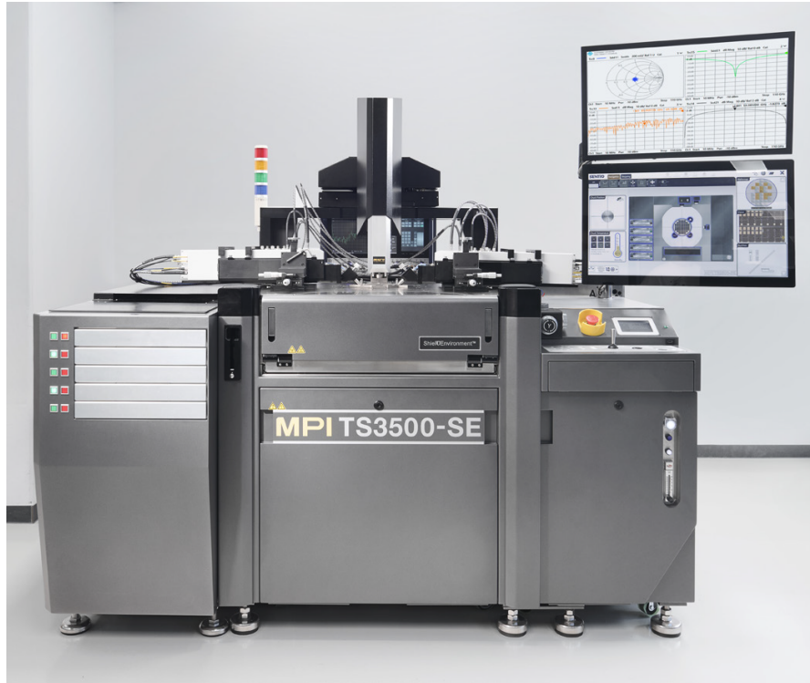
Integrated system for differential mmW characterization with R&S(R)ZNA Vector Network Analyzer and MPI TS350-SE Fully-Automated Probe System
